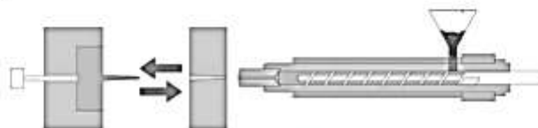
Figure 1.9 Injection moulding: mould open
